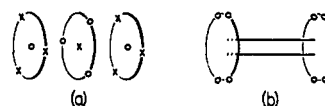
Figure 54.—Representations of the electronic structure of oxygen: (a) spin sets anticoincident; (b) spin sets coincident.
